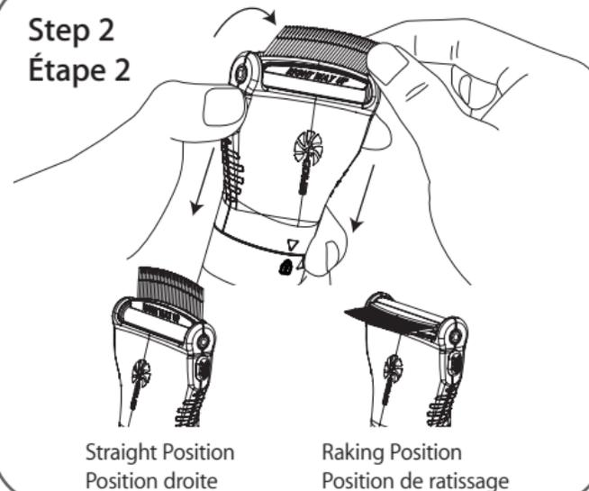
Push and hold down the knobs on both sides to manually adjust the combing angle. Two set positions are available: straight or raking position.
