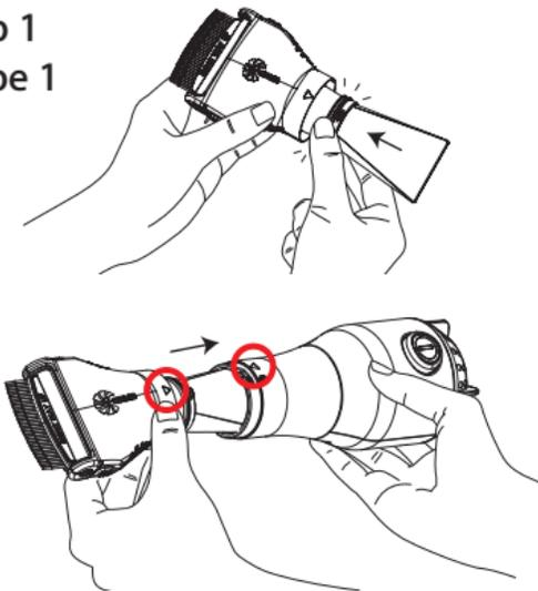
Securely attach a capture filter to the V-Comb combing head, ensuring it clips into place (until you hear a click). Re-attach the combing head to the main body by aligning the guiding arrows and twist to lock.
